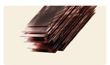
Our cathodes are made of pure copper with a copper content of at least 99.99%. The main impurity is silver (6 to 10 ppm). Brixlegg cathodes are registered on the London Metal Exchange (LME) under the "BRX" brand as "Cathodes Grade A." They comply with the EN 1978 standard, the IWCC requirements, and ASTM B115.
