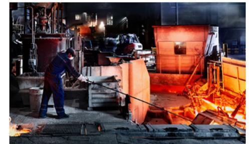
ANODE FURNACE WITH CASTING
