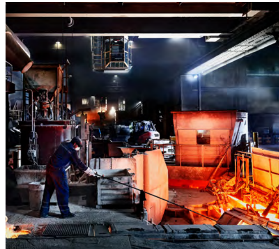
ANODE FURNACE WITH CASTING LINE
